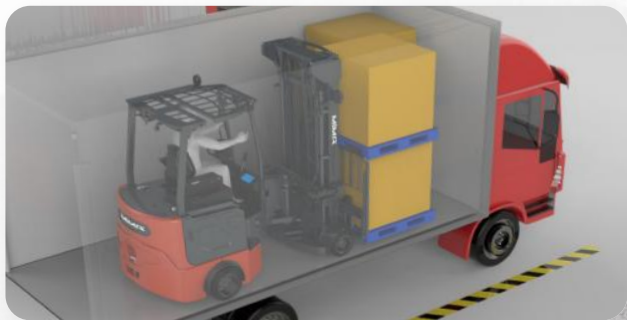
Low mast design enables handling inside containers
